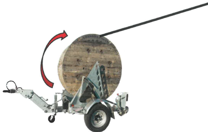
Figure 14: Rotation direction of drum
