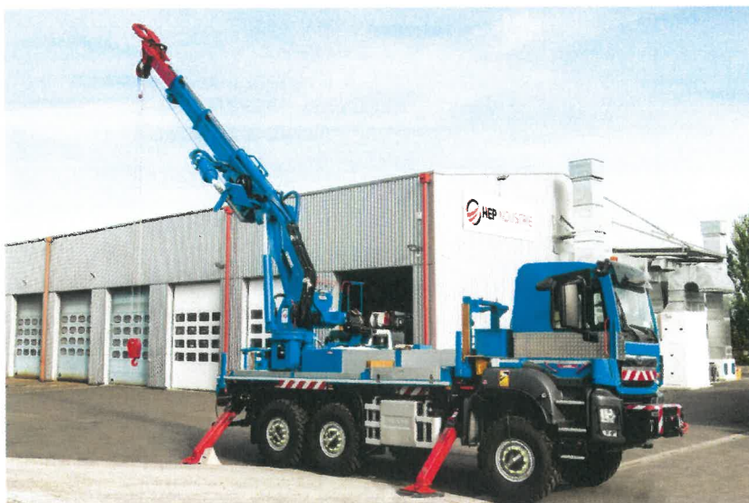
Vehicle and crane that can be used for live line work pole erection
